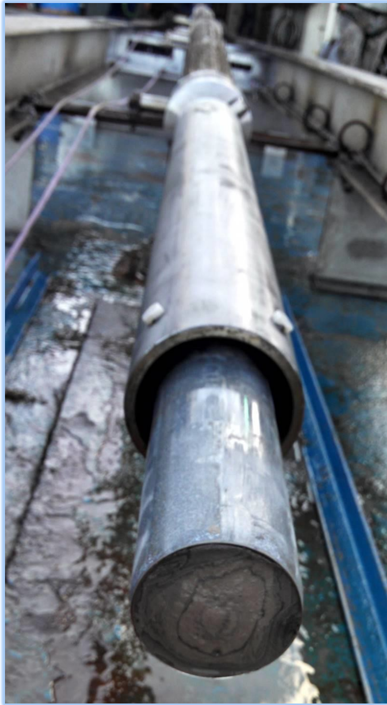
Figure 28) Photo Of The Stinger Sampler Shelby Tube With A Soil Sample From 40 M Depth
