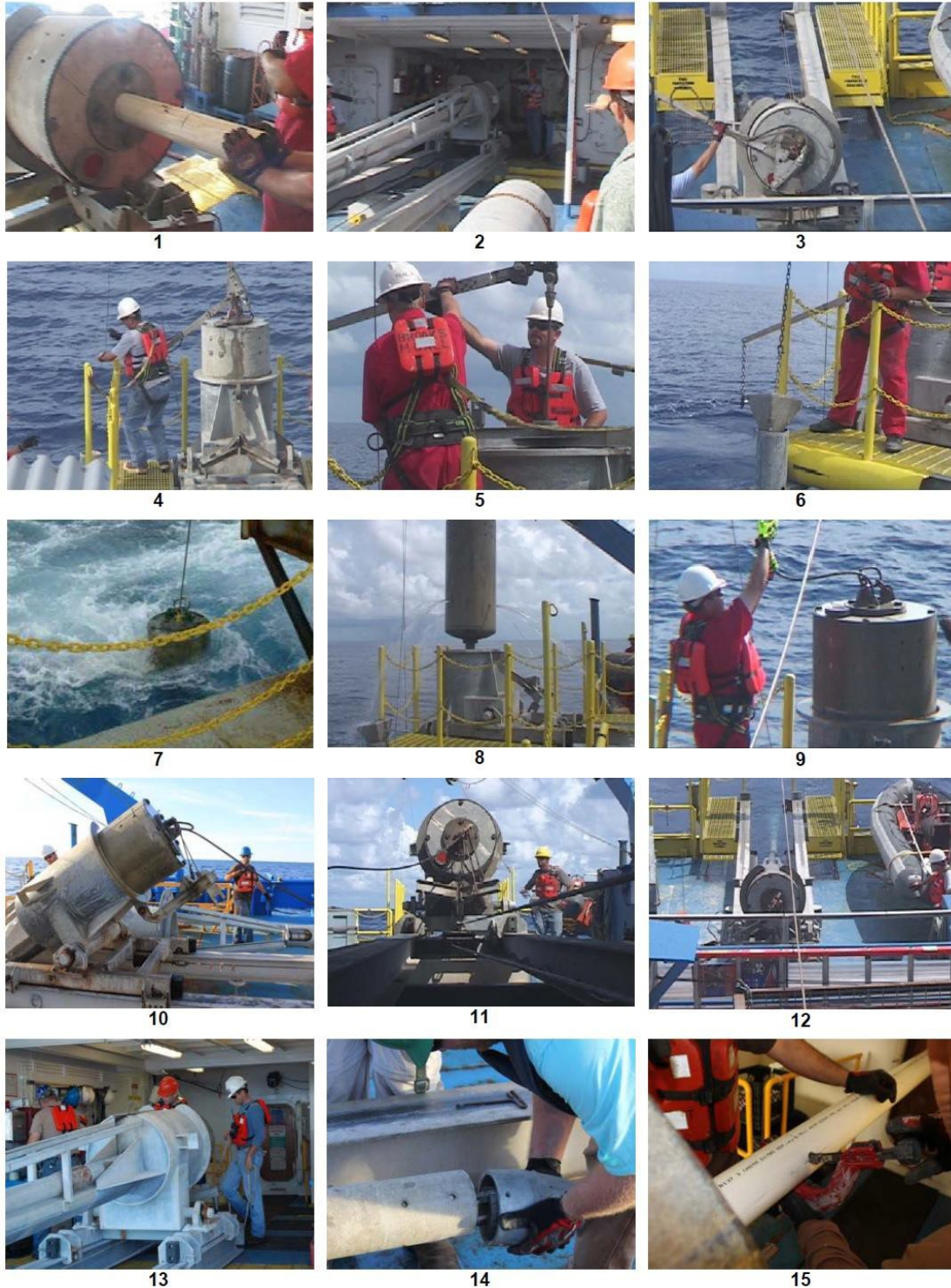
Figure 18) Stepwise Process Of JPC Operations
