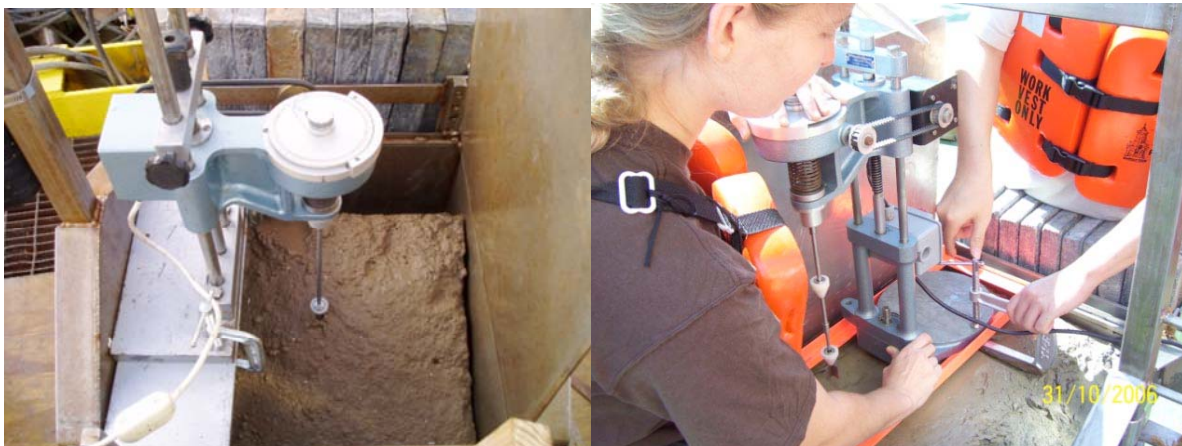
Figure 3. Shear strength testing down 50-cm x 50-cm large box cores.
