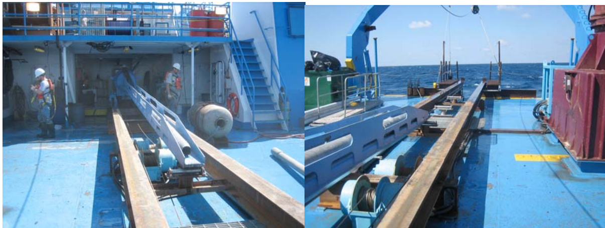
Figure 2. Jumbo Piston Coring (JPC) rigging on the R/V BROOKS McCALL.
