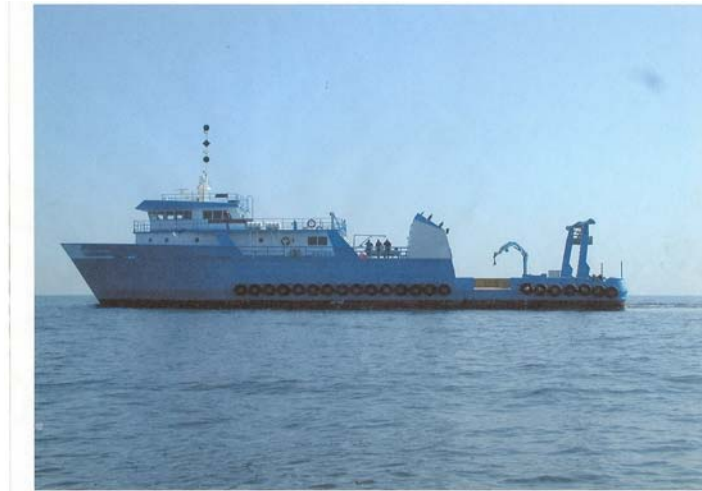
Figure 1. The R/V BROOKS McCALL that TDI-Brooks has outfitted for geotechnical coring, including Jumbo Piston Coring in the Gulf of Mexico.
